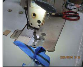
Photo of non-conformity NC No finger protection guard for the sewing machine.JPG
