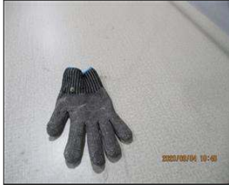
Photo of the personal protection equipments (if applicable) Metal glove for the cutting worker.JPG
